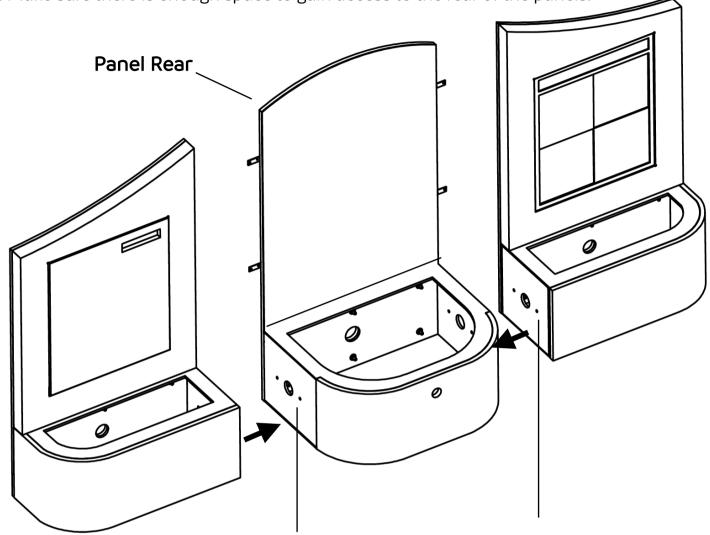
**5)** Place the M12 bolts, washers and nuts through the side of the platforms using the holes and tighten using the wrench.
