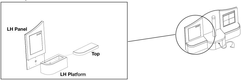
**2** ) Identify - LH Light Panel and place it to the Platform. Use 6 x M12 bolts - 6 x M12 washers and attach the Platform to the wall panel through the aligned 6 holes.
