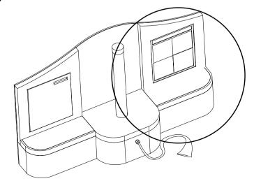
The Mirror Panel and the Center Platform are a little larger. The process of attaching them together is exactly the same as the LH and RH side of the sensory station. The mirror section includes key equipment and the cord management.
