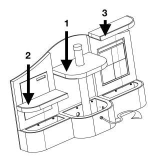
11) Fit all three platform tops starting in the middle. You may have to jiggle the Bubble Tube / Waterless Column a little to make sure it stands upright on the base.
