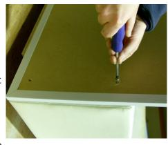
and side properly aligned, drive two screws through the pre-drilled holes and into the side of the platform (top left, bottom right). Do not install the remaining screws until the second mirror is installed and in alignment.
