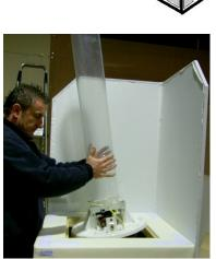
9. Place the transformer into the base. and plug the XLR connector (right) into the bubble tube base. Run the power cord out of the hole in the bottom of the platform. Replace the lids and secure with the previously removed screws.
